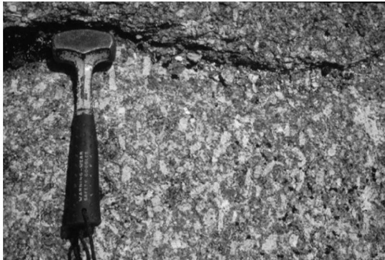
Fig. 4. Photograph of the Mount Waldo granite on a glacially polished surface. 2 lb crack hammer for scale. Potassium feldspar phenocrysts are the aligned white tabular minerals. Foliation defined by these feldspars is magmatic in origin and ubiquitous in the pluton.
